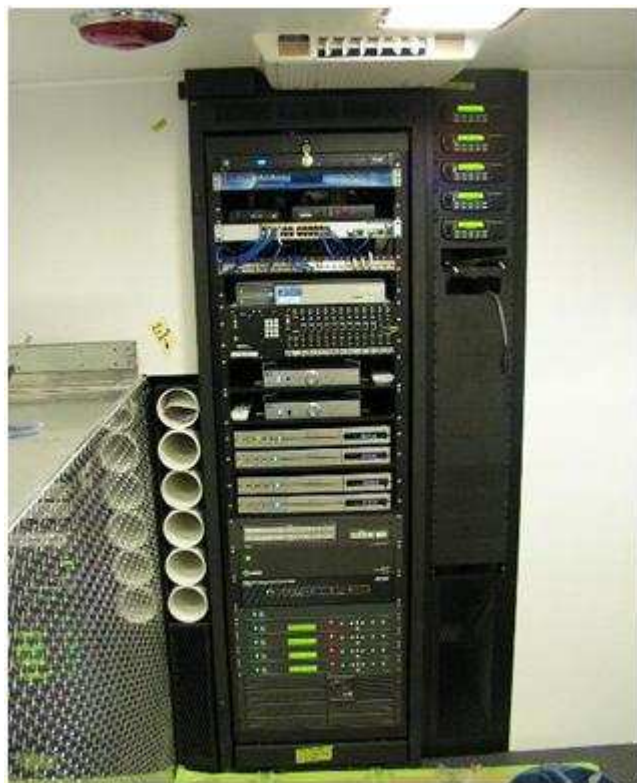
Figure 8 Typical SVI Truck Equipment Rack Including Support for Voice, Data, Video and Radio Interoperability via a ACU-1000 Gateway
